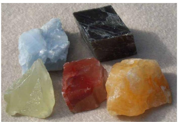
It is transparent to opaque, with occasional phosphorescence or fluorescence. Icelandic spar, a transparent variety, is used for optical purposes. Single calcite crystals have an optical property called birefringence, which is double refraction. It
