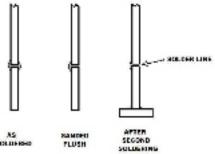
To avoid this when I have another soldering operation to follow, I try to leave a little extra solder on my joints. For instance, when trimming off excess base plate from around a bezel, I leave a couple paper thicknesses excess plate material whenever possible until I'm done with all soldering. Of course, this isn't always possible as when a soldering operation would prevent you from gaining access for final sanding and polishing of an area.
