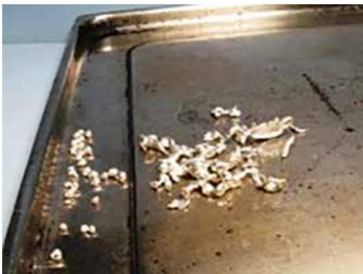
But there's an easier way to get a good supply of balls. Some casting grain comes in near perfect ball form. Just grab your tweezers and pick out the ones you need. When you need larger quantities of balls, pour the casting grain out onto a baking pan, tilt the
