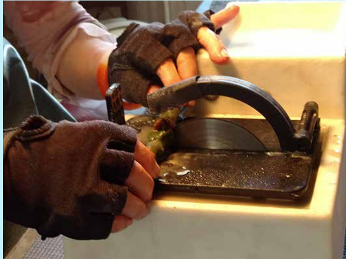
Diana St. John cuts agate hearts using dop sticks to hold the stones.
